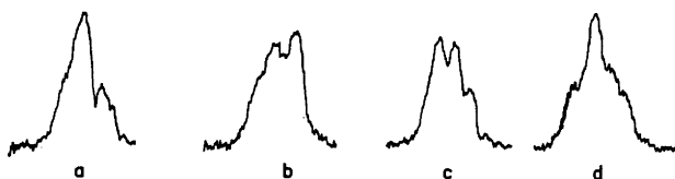
Fig. 11. The results of the double resonance experiments in N-(2-furfurylidene)aniline (a–d) show the H\alpha band for selective decoupling of J_{H\alpha-4} . The corresponding positions of the decoupling field are indicated by arrows in Fig. 9.
